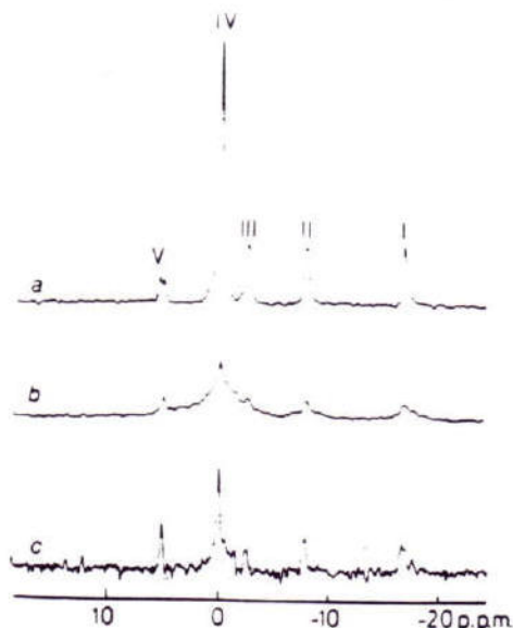
Fig. 2 ^{31}\text{P} -NMR spectrum of a two-compartment phantom containing ATP (signals I, II and III), phosphocreatine (IV) and inorganic phosphate (V). A single-turn saddle-shaped radio-frequency coil operating at 73.8 MHz was used in a standard wide-bore (89 mm) superconducting magnet. Profiling was obtained with a coil system designed to provide spatial localization across an internal volume ( 2\sigma \sim 15\text{--}45\text{ mm} ) whilst maintaining a homogeneity of \sim 0.1\text{ p.p.m.} at an operating B_0 field of 4.3 T. The working bore of the system was 45 mm. The spherical compartment contained 4.65 mM ATP, 9.30 mM PCr and 3.72 mM \text{P}_i , and the cylindrical compartment contained 4.65 mM ATP, 18.60 mM PCr and 1.86 mM \text{P}_i . a , Spectrum (300 scans) in the absence of localizing fields. A 6-Hz line broadening exponential multiplication was used to enhance the signal-to-noise ratio. b , Spectrum (600 scans) with the axial extent reduced to 20 mm. The same line broadening was used as in a . c , Spectrum obtained on removing the broad component of spectrum b by convolution difference 9 . Line broadenings of 6 and 60 Hz were used and the vertical scale in the spectrum was multiplied by 4 for clarity of presentation. Chemical shifts are defined as positive in the high-frequency direction with phosphocreatine taken as an internal reference.
