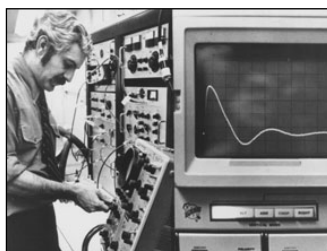
THE DISCOVERY THAT MADE MRI HAPPEN. Dr. Damadian with the NMR instrument he used to discover the cancer-detecting MR signal.
